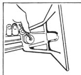
1. On the underside of the Pattern Matcher is a black Allen screw holding a "cup" washer and the powerhead in place. Remove the black Allen screw with the Allen wrench provided.
