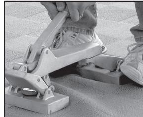
2. Use the Nap Grip head dial to properly adjust pin penetration into only the carpet backing and not into the carpet padding. This will reduce the risk of carpet damage and ensure proper stretching.
