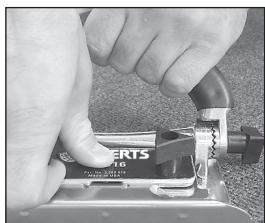
2. Disengage the teeth and adjust to desired setting. Re-tighten the knob firmly.
