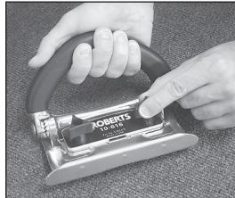
4. Tighten knobs firmly to secure blade holder.
