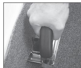
3. Move the trimmer in the opposite direction to complete the cut at the corner.
