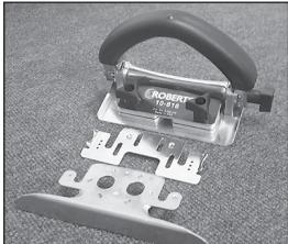
1. Three basic parts of your Trimmer: (Top to Bottom) Product Body, locating plate and blade holder unit.
