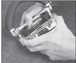
2. Insert locating plate between spacers at the height desired, using the finger notches at either end. The average location will be on top of the fourth spacer. If this leaves the carpet too long move down one or two spaces. If the carpet is too short, move the locating plate, to a higher position.
