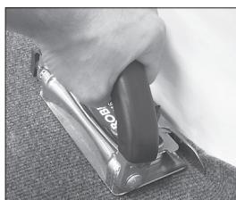
4. Optional: Using the guide bar, tuck the carpet into the gully to complete the job. The large handle will permit you to use both hands when necessary.
