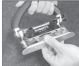
3. Insert the blade holder above the locating plate. Adjust "in and out" dimension for type of carpet being trimmed. There are three positions. Make sure both sides of the plate are on the same position.
