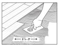
NOTE: Never work on top of the flooring when installing. If you must work on top of the newly laid flooring, use a kneeling board.
