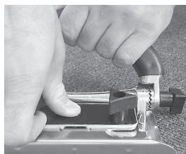
2. Squeeze the handle to open up the handle and disengage the teeth. Re-tighten the knob firmly after setting handle to the desired angle.
