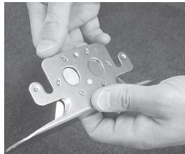
The blade-holder unit has two "finger holes" to facilitate removal and replacement of blade.
