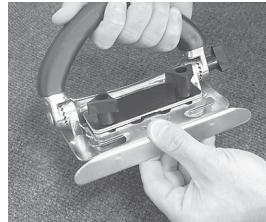
3. Insert the blade holder above the locating plate. Adjust "in and out" dimension for type of carpet being trimmed.
