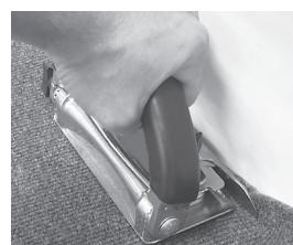
4. Using the guide bar, tuck the carpet into the gully to complete the job. The large handle will permit you to use both hands when necessary.
