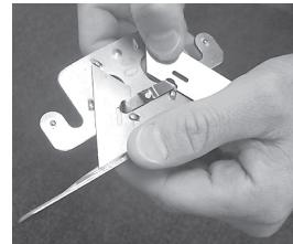
Remove old blades as shown. Insert new blade under spring clip and position between raised guides. When only one end of each blade is dull you need only switch blades to the other position to double the life of the blades. For satisfactory performance, you must be able to read the printing on the blade, when it is in position.
