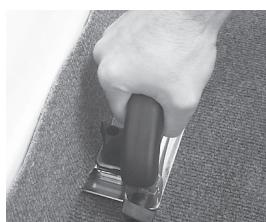
2. Keeping the base plate flat on the carpet and the guide bar against the wall, make the trimming cut.
