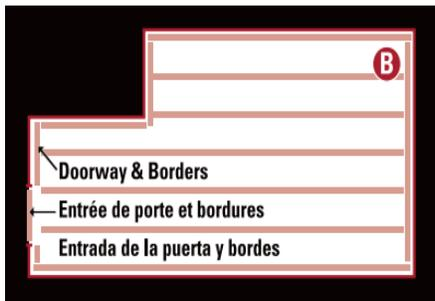
Placement Recommendation: Apply strips to the perimeter of the room, down the center, along doorways and across the interior of the room (see B). Always follow the floor manufacturer's specific installation guidelines.
