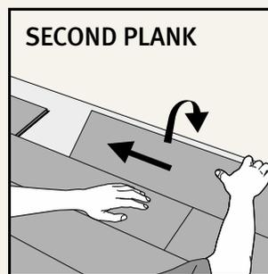
**2** Angle the long side groove of the second plank into position at the tongue of the adjacent plank from the previous row and fold down. Now slide the second plank to the left to position it to the right short side of the first plank. Press down firmly and listen for the click that means it's locked in place.
