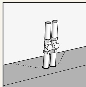
Mark the center point of the pipes on the plank. If the required expansion gap is 10mm, drill holes 20mm bigger than the pipe diameter. Cut as shown below. Apply white glue and install the floor pieces. Cover the holes with pipe collars or fill with a joint sealer.
