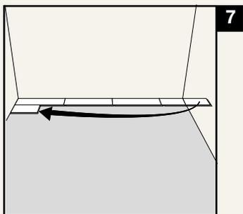
To begin the second row, use the remainder of the cut plank you used to finish the first row.
