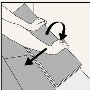
**1** When installing in reverse, start from the left. Angle the long side groove into position at the tongue of the adjacent plank from the previous row and fold down to lock into place.
