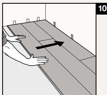
Continue to install the row as before. When you have completed 2–3 rows insert wedges between the wall and the first row so there is a gap at least ½" (8-10mm) wide.
