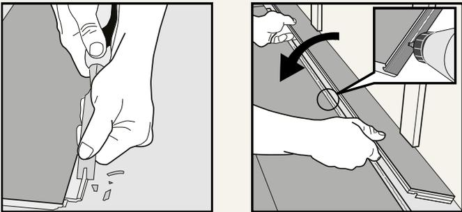
Remove the locking element/hook as shown in the diagram. Use white PVAc glue to connect the planks. Press/place wedges between the glued strip and the wall.
