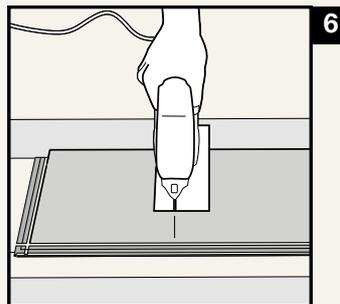
Cut the row’s last plank to size. If you are using a jigsaw, cut it face down. If you are using a hand saw, cut it face up.
