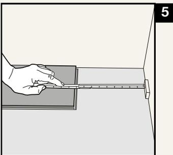
Continue installing the first row. When you are close to the wall on the right side, place a wedge at the wall and measure the length to determine the size of the row’s last plank.
