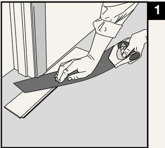
Door frames can be removed and raised, but it’s usually easier to cut them. Use a loose plank as a template and saw off the excess. Ensure that the floor is not pressed between the subfloor and the door frame.
