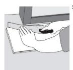
12) You can undercut door frames by turning a panel upside down and using a handsaw to cut away the necessary height so that panels slide easily under the frames.
