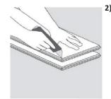
Remove the tongue, on the long side of the planks that face the wall on your first row. This is to ensure that the decorative surface of the flooring is well under the finished trim when installed. Use a utility knife to score through the tongue several times until it easily snaps off. Seal the cut edges with a silicone sealant.
