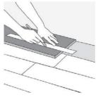
10) To fit the last row, lay a plank on top of the previous row. With the tongue to the wall, lay another plank upside down on the one to be measured and use it as a straight edge. Don't forget to allow room for the expansion spacers. Cut the plank and attach into position.
